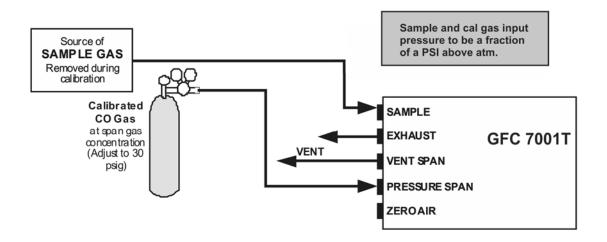
Figure 9-6: Pneumatic Connections – Option 50E: Zero/Span Calibration Valves
